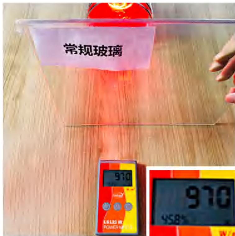
Under the same light source, normal auto glass, the light intensity value is 970, the infrared rejection rate is 54.2%.
