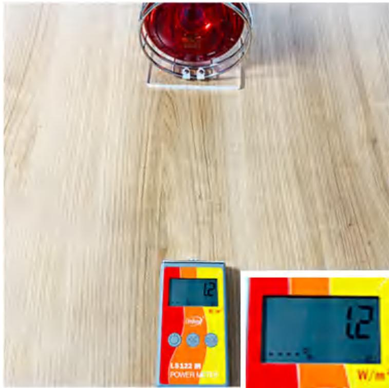
measuring instrument on, the light intensity value is 12.
